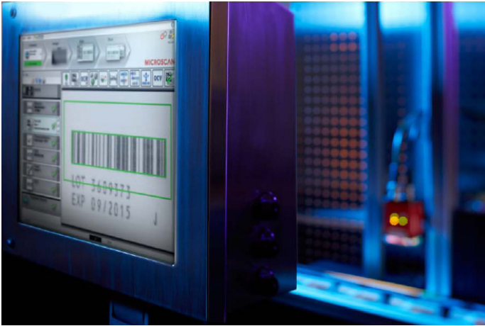
Figure 13: A machine vision system grades the print quality of a barcode applied to packaging and monitors for any trending degradation in the print process.
