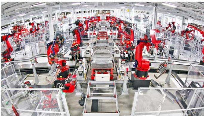
Figure 5: An automotive manufacturing facility uses a highly-sophisticated network of sensors and robotics, which send and receive data across the factory floor to fully automate vehicle assembly.
